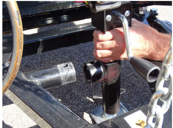
4. Remove crankstand from a-frame.
