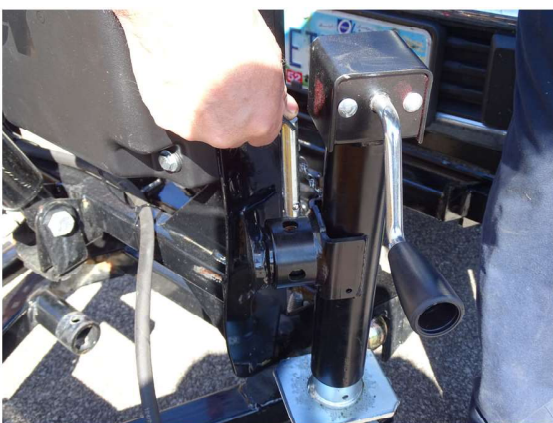
5. Attach crankstand to lift frame.
