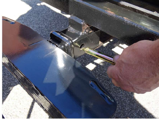
2. Install receiver hitch pin and hair pin.
