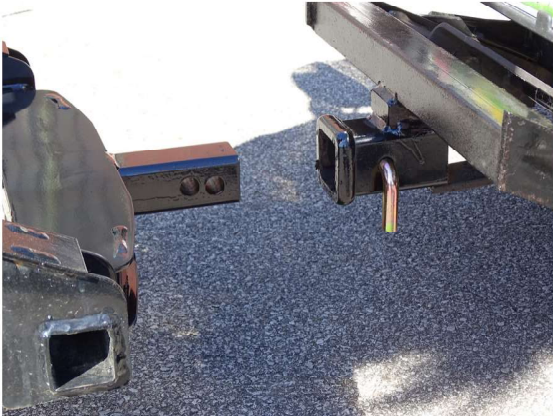
1. Pull vehicle into plow assembly and push plow assembly forward an inch or two.
