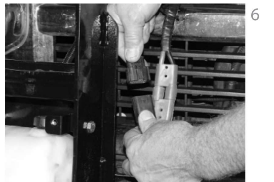
6. Remove weather covers and connect both electrical plugs.
